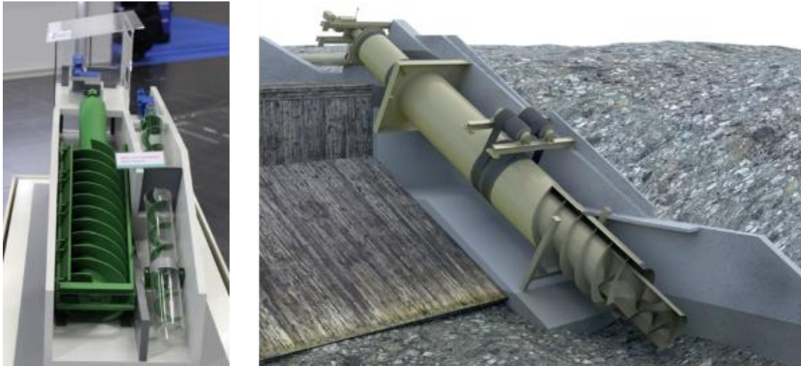
Figure 45: A parallel Archimedes screw set by Rehart Power (left) and a 3D view of Hydroconnect coaxial screw unit (right) at the RENEXPO Interhydro Fair in 2017 (source: J. Steller)
