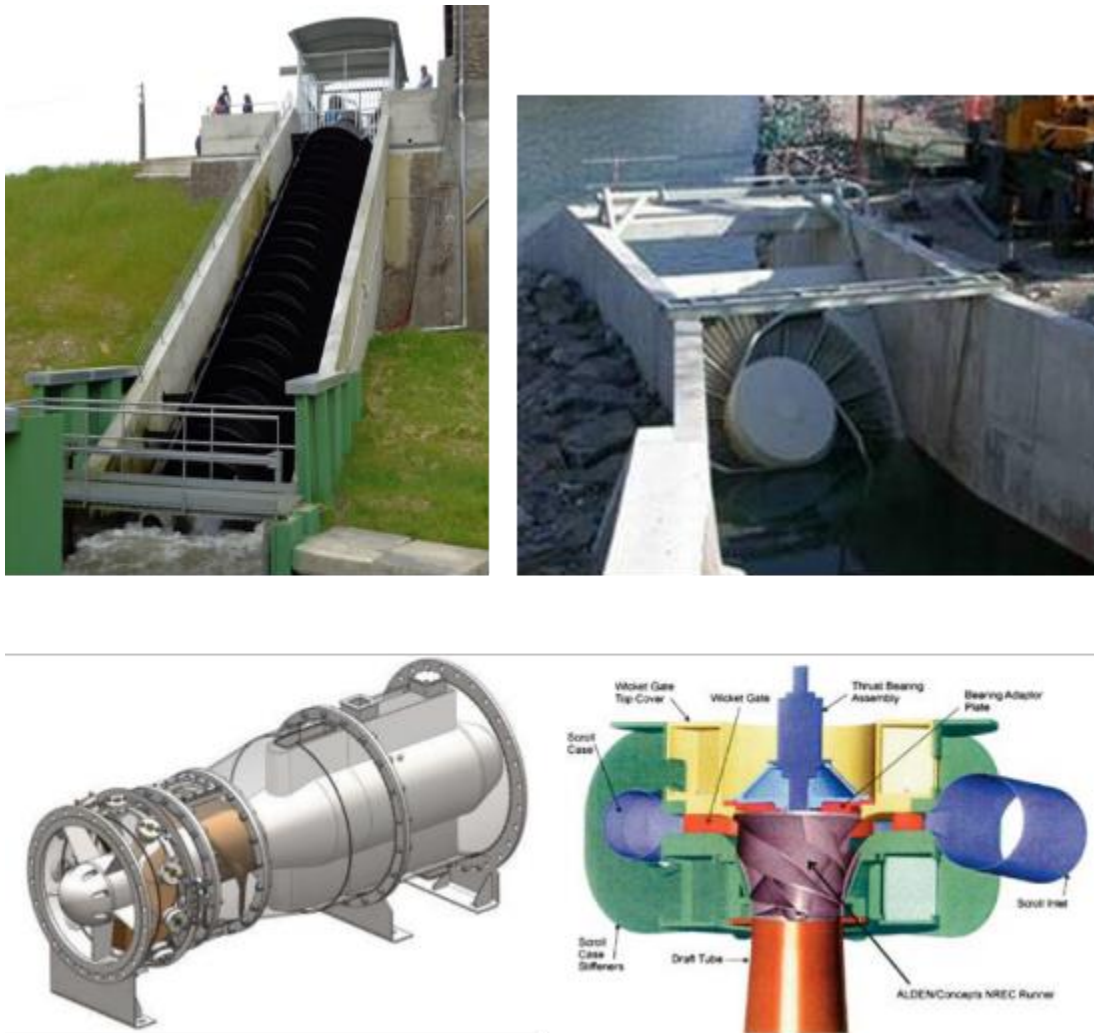
Figure 82: View of fish-friendly turbines: screw (up left), VLH (up right) (source: MJ2 technologies), Pentair fair-banks (down left) and Alden turbine (down right)
