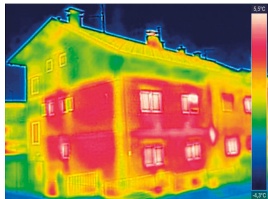
Thermal imaging of a home's exterior reveals its 'hot' and 'cold' spots. Here, walls and windows (red areas) are letting warm air escape while the roof area shows better capacity to keep heat in. Notably, there are no blue areas in this photo, which would identify where insulation is working effectively. Photo: iStock / Ivansmuk.
